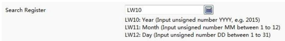
The screenshot shows the "Search Register" configuration interface. It features a label "Search Register" on the left and a text input field containing "LW10" with a calendar icon on the right. Below the input field, three lines of text provide instructions: "LW10: Year (Input unsigned number YYYY, e.g. 2015)", "LW11: Month (Input unsigned number MM between 1 to 12)", and "LW12: Day (Input unsigned number DD between 1 to 31)".
