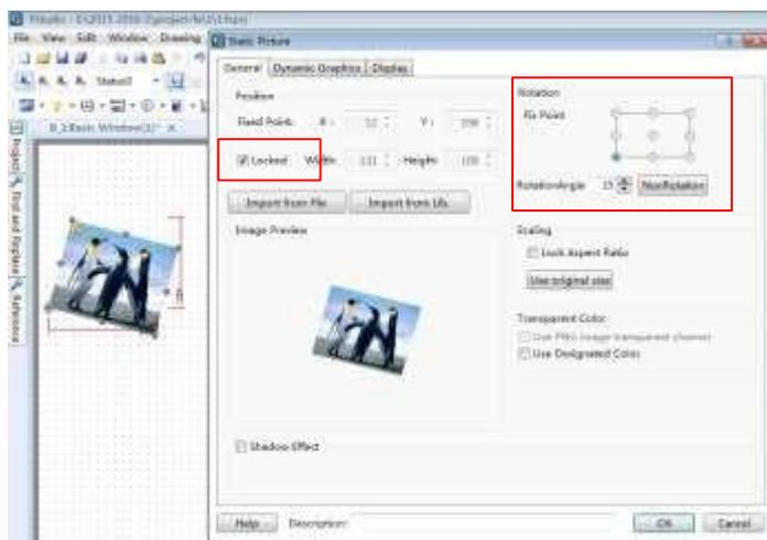
The static picture size can be set in the properties window by the Scaling function. It can be set either by checking “Lock Aspect Ratio” (the fixed horizontal/vertical ratio) or by checking “Use original size” (keeping the original size).
