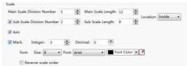
You can set the “Main Scale Division Number”, the “Main Scale Length” and the “Sub Scale Length” here. The Location of the scale can be set “Inside”, “Outside” and “Center”, as shown as below. The “Sub Scale Division Number” and the “Axis” are checked by default. The default sub scale division number is 2. If the “Sub Scale Division Number” and the “Axis” are unchecked, that means the sub scale and axis are not displayed.
