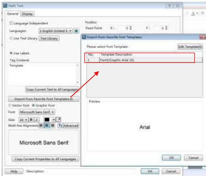
First, click the button "Import from Favorite Font Templates" in the property window of a Static Text component to open the "Import from Favorite Font Templates" dialog. Then select the required font template and click the OK button. The result is shown as below.
