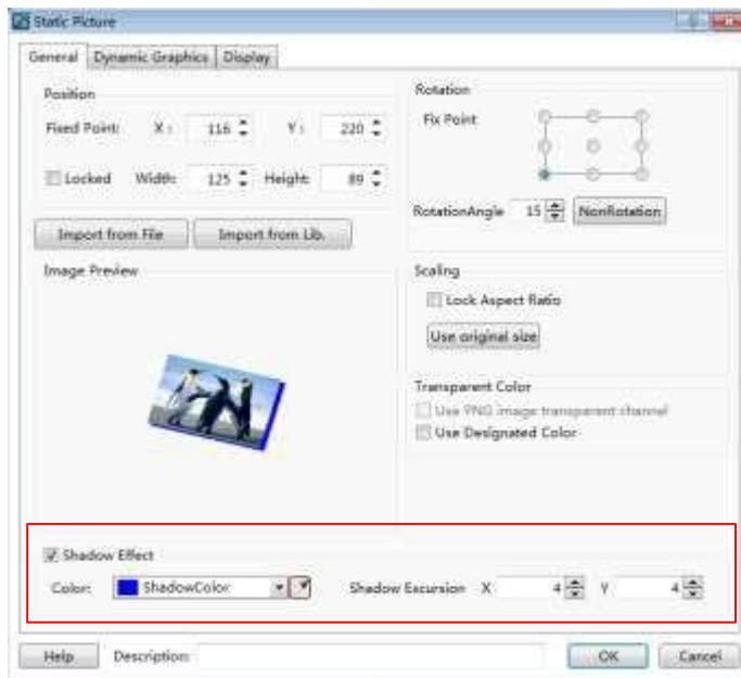
The static picture can be set to display only when the corresponding conditions are satisfied. The user can choose that the static picture is displayed all the time or displayed in conditions by setting the Display properties. The conditional display type includes Level User, Privilege User and Logic Control.
